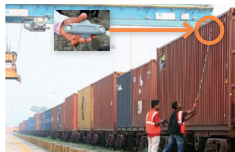
RFID easily attachable to container using magnets
