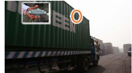
RFID easily attachable to container using magnets
