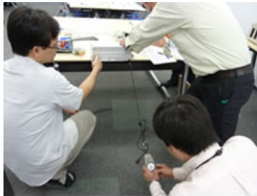
Testing the strength of a locked power cable at Safety Review Workshop
