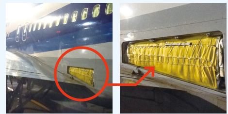
Boeing 767 With Missing Panel
