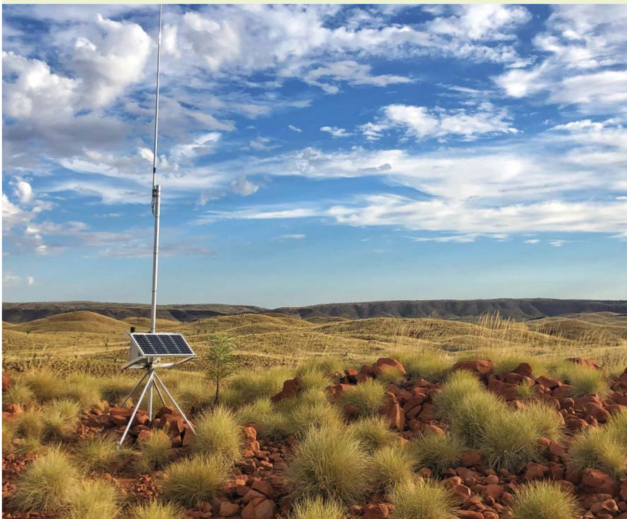
Motus towers used to track Ghost Bats, Pilbara Leaf-nosed Bats and Northern Quolls. Photo: Brendan Stratton, BHP.
