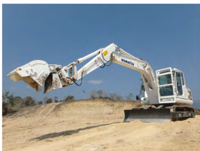
Machine developed based on hydraulic excavator (for processing unexploded ordnance)
