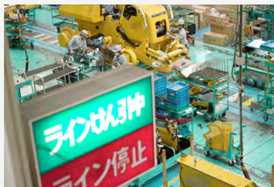
Assembly work on rotating assembly line floor panels
