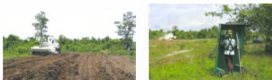
(left) Komatsu's demining machine for anti-personnel landmines rotates rollers with spikes attached (rotary cutters) to crush and explode anti-personnel landmines in the ground. It operates over a large area of land, tearing up bushes and weeds and transforming the land to look as if it were a field (Cambodia, 2006).
