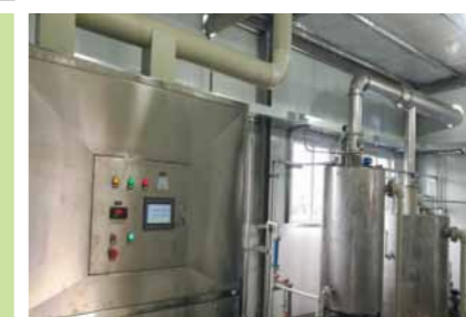
◀ CWPO microwave wet catalytic oxidation technology
