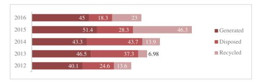
The generation of carbon lining waste during the reporting period decreased by 12% compared to 2015 and made up 45 thousand tonnes. The quantity of processed waste dropped twice compared to the previous period. Since 2014, secondary raw materials obtained from recycling have been sold to the West Siberian metallurgical plant.
