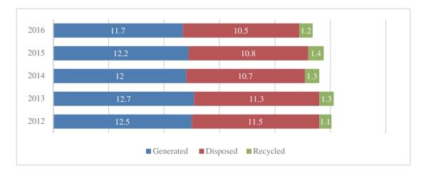
The quantity of processed mud is directly dependent on the implementation of the measures for the construction of red mud disposal areas. In 2016, the level of generation of mud from alumina production reduced to 11.7 million tonnes, the volume of mud recycling also reduced to 1.2 million tonnes.
