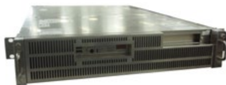
A rack-mountable RS90 series of information and control server.
