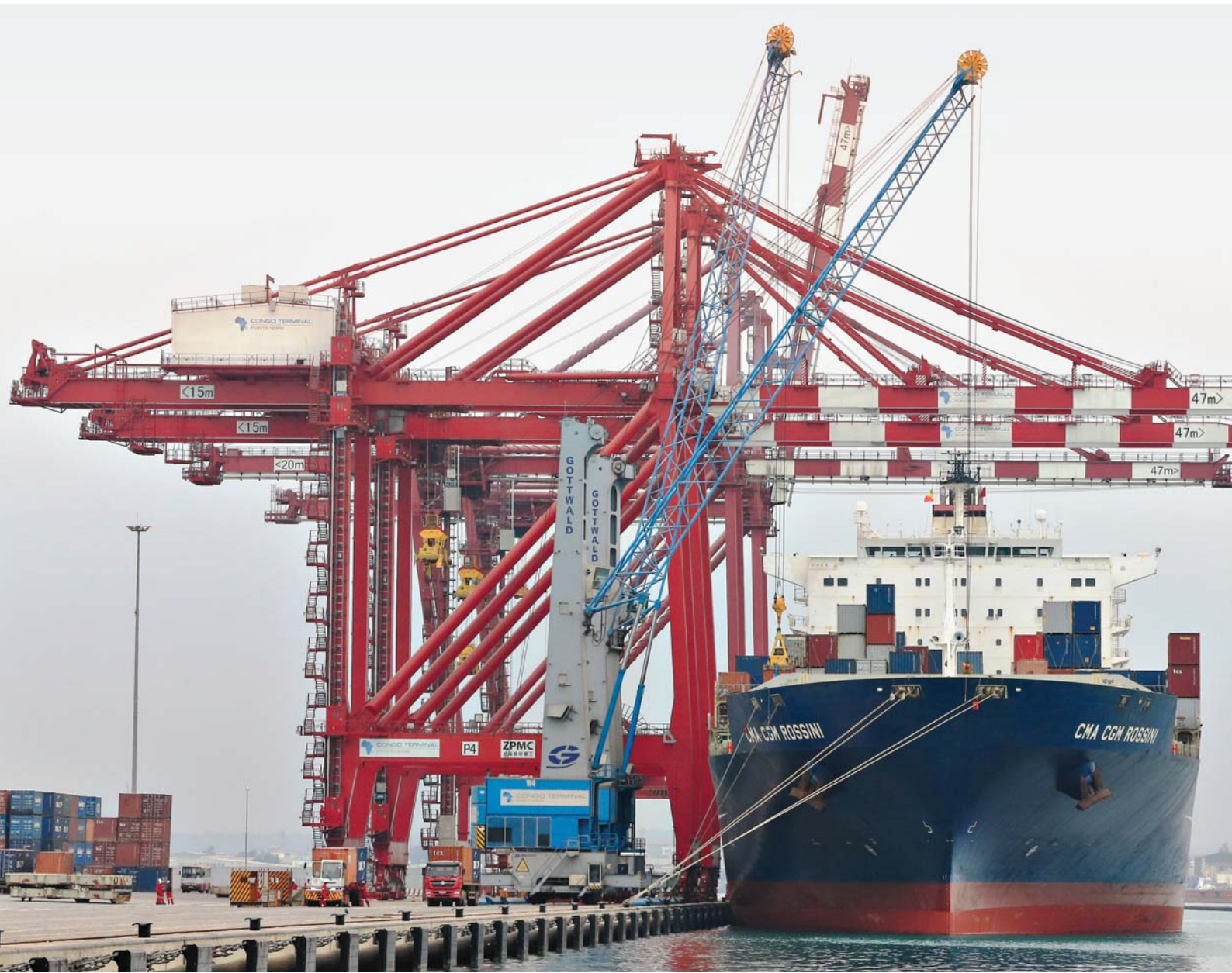
Port concessions Congo Terminal at Pointe-Noire, with six gantries capable of handling ships with 16,000-container capacity. —
