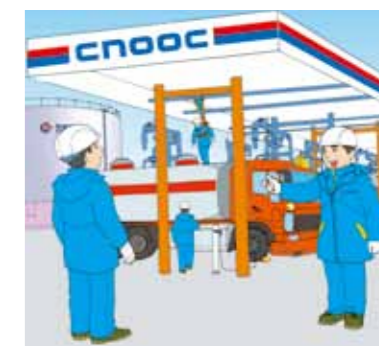
The engine of the truck must be shut off and electrostatic clamps must be used
