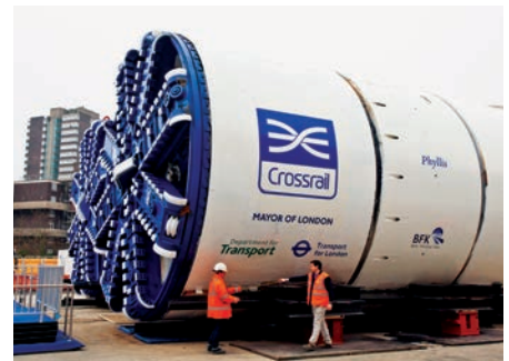
Crossrail tunnel boring machines
