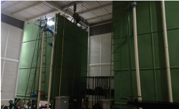
The fully automated biogas plant in Bengaluru campus has a capacity of treating two tonnes of food waste per day
