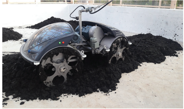
The solar-heat assisted automated sludge dryer has a cumulative treating capacity of 1.2 million kg of sludge per year
