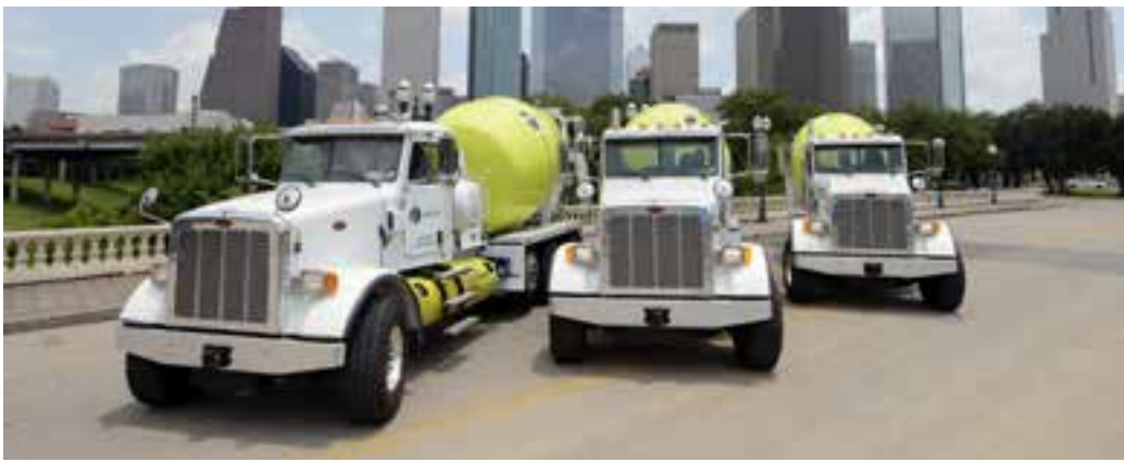
Compressed natural gas powered mixer in Houston, USA Region
