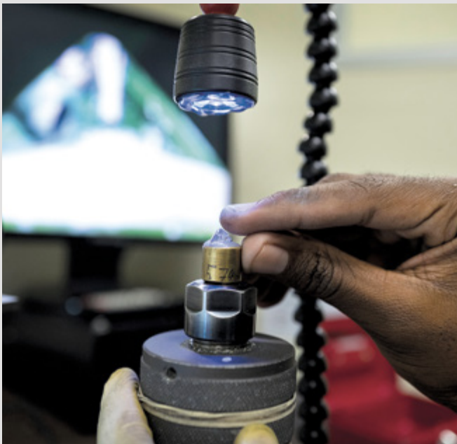
Sightholder examining a De Beers diamond as part of the cutting and polishing process, Gaborone, Botswana.
