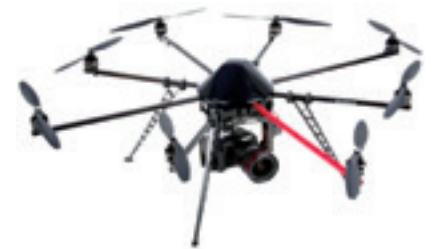
Drone: Equipped with thermal imaging and video camera
