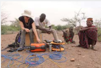
Advisian geophysicist performing an electrical resistivity tomography survey to find new groundwater sources.
