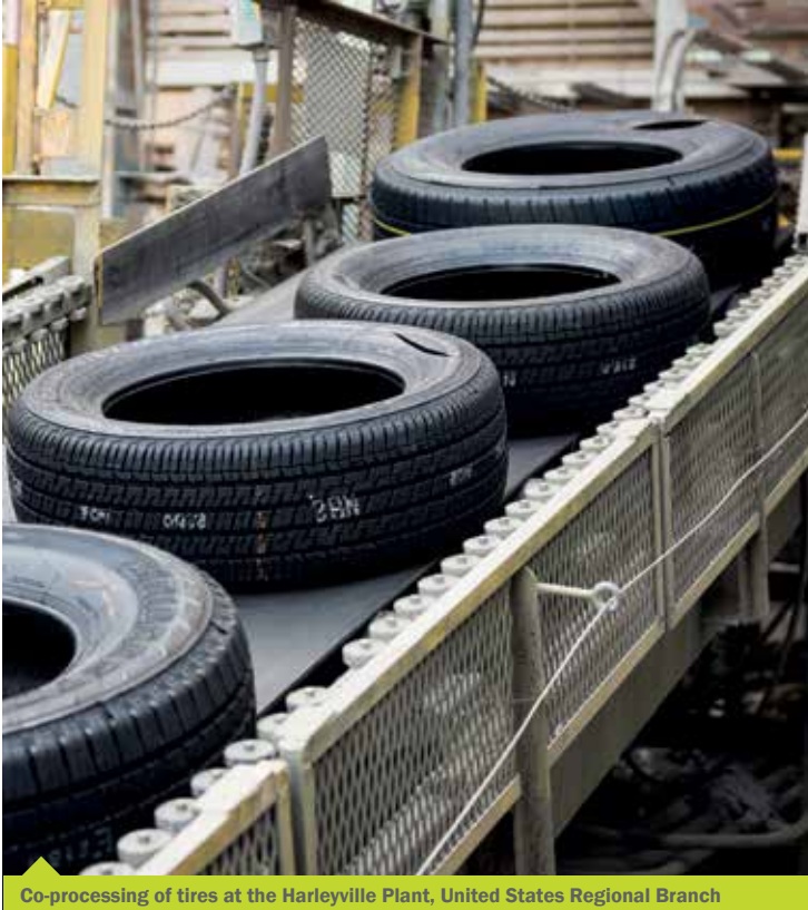
Co-processing of tires at the Harleyville Plant, United States Regional Branch
