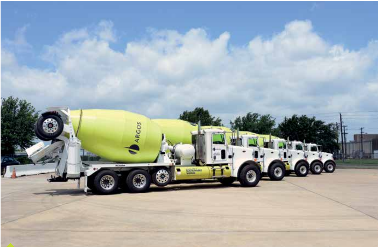
Cement mixing trucks that run on natural gas, United States Regional Branch
