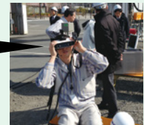
When users look through the head-mounted display, the image of the completed building appears superimposed on the unfinished construction site
