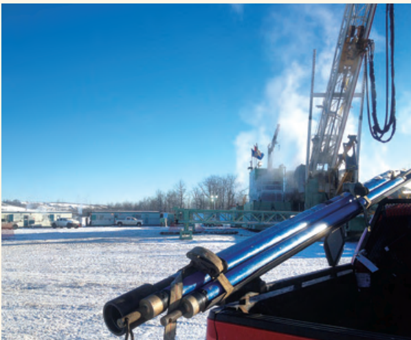
Easy-PCL horizontal well tool is used for well logging in Canada.
