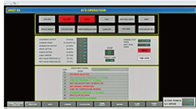
Automatic turbine startup window
