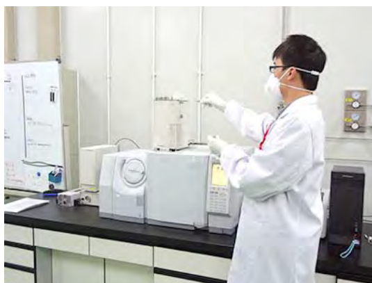
This high-precision analyzer verifies that plastic components do not contain restricted chemicals.
