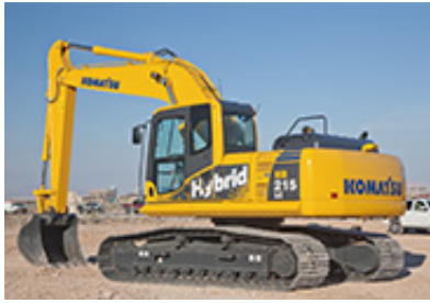
Hybrid excavator that have 25% higher efficiency than conventional vehicles
