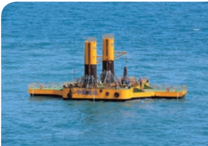
Offshore tidal power generation unit
