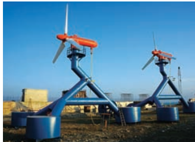
Onshore tidal power generation unit
