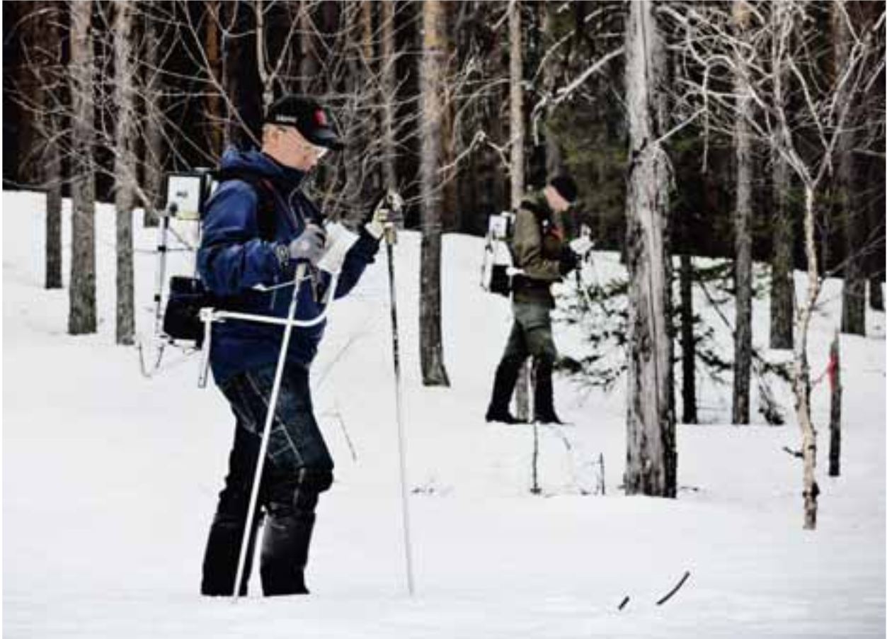
Survey technicians at Boliden, collect geophysical data during a so-called electromagnetic measurement survey. Deposits can be discovered at up to around 1 km's depth under the surface with the aid of Boliden's in-house developed electromagnetic method.
