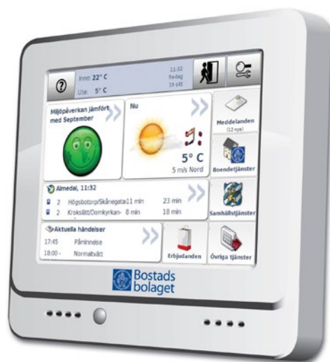
This BoVist information unit enables tenants to book laundry times, receive information from Bostadsbolaget and monitor their own energy consumption.
