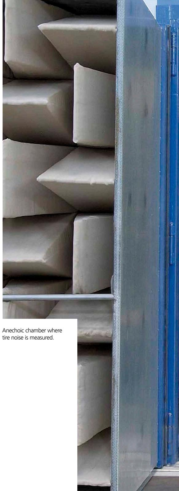
A photograph of an anechoic chamber, showing a series of large, grey, pyramidal-shaped electromagnetic wave absorbers arranged in a grid pattern. The chamber's walls are blue, and the lighting is focused on the absorbers, creating a sense of depth and texture.
