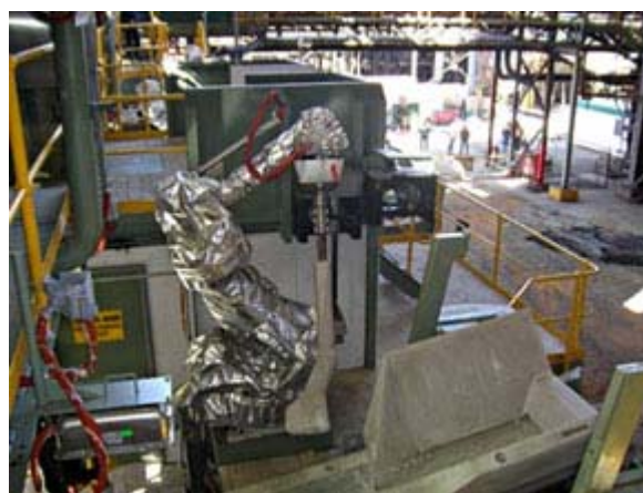
Remotely operated robot used to manage the presence of a crust.
