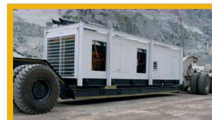
A Cat powered Motivator mobile generator, designed to provide in-pit mobility for the relocation of electrically powered mining plant, such as shovels.
