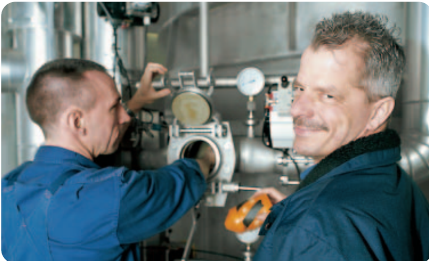
Jens G. Larsen and Keld Johnsen in Kalundborg with a novel cleaning device invented by employees to improve cooling efficiency in fermentation tanks resulting in major environmental and financial gains.
