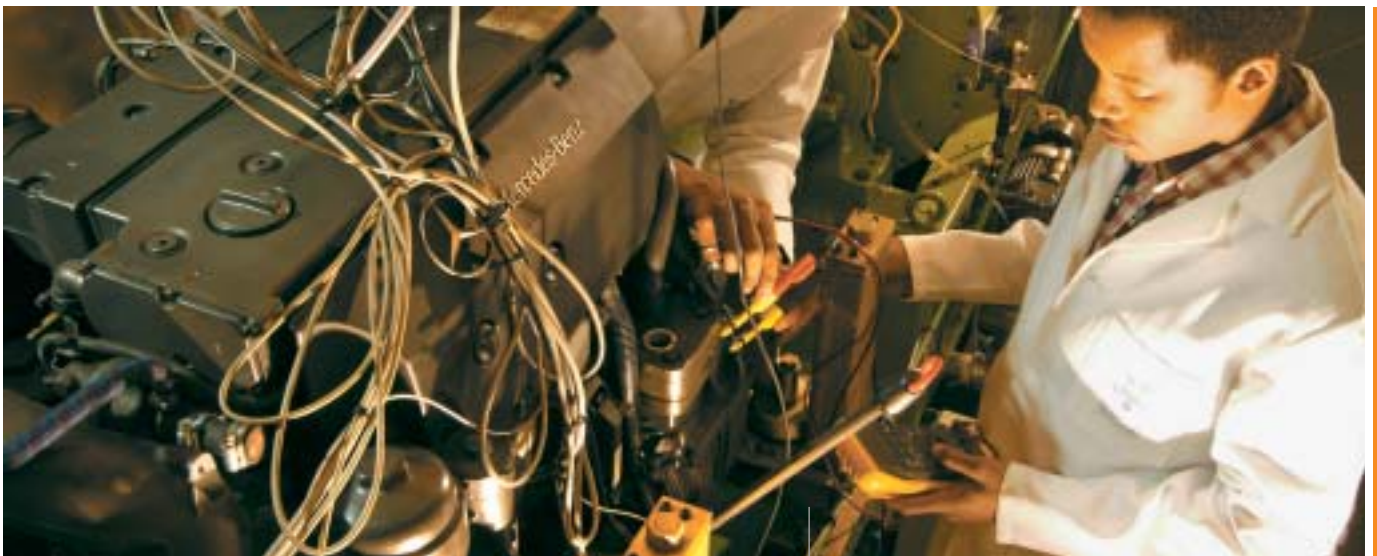
Testing Sasol-developed diesel on a test engine at Sasolburg
