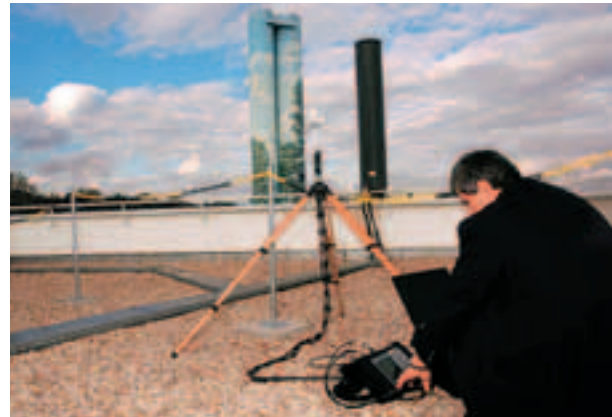
▲ Measurement of electromagnetic fields on site.
