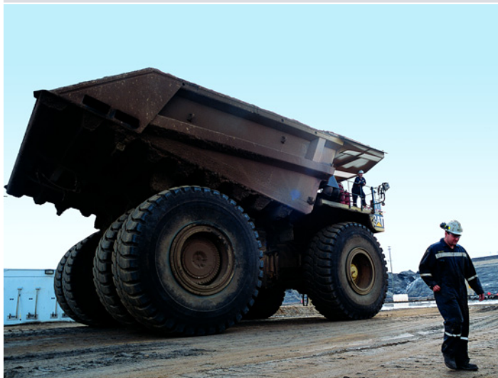
Athabasca Oil Sands Project truck which has the capacity to carry 400 tonnes in one load
