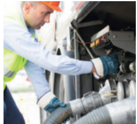
▲ A tanker driver connects a tank to a loading hose at a BP service station in Turkey.
