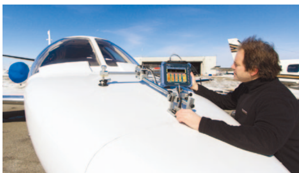
An engineer checks the interior of CFRP materials using an ultrasonic phased array flaw detector.
