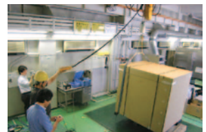
Packaging is subjected to a dropping test.
