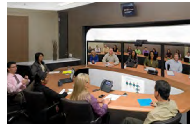
Cisco TelePresence CTS-3000 unit (6 users) connecting with a TelePresence CTS-3200 unit (18 users)
