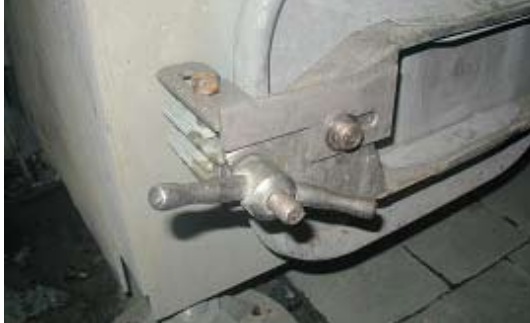
Some of the hatch modifications introduced after the Povolze, Russia fatality.
