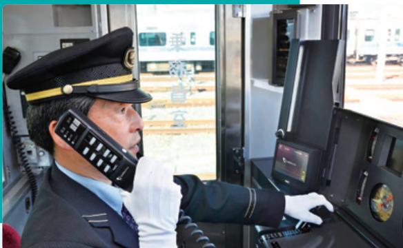
NEC's digital train wireless system for Odakyu Electric Railway
