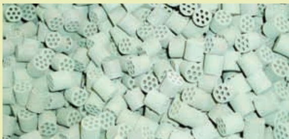
Yara's N 2 O abatement catalyst can reduce GHG emissions substantially.
