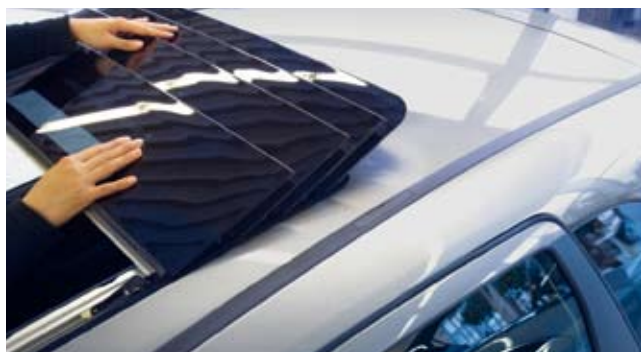
Innovation in automotive engineering: The Makrolon® sunroof
