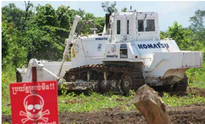
●● Komatsu demining machine for removal of anti-personnel mines
