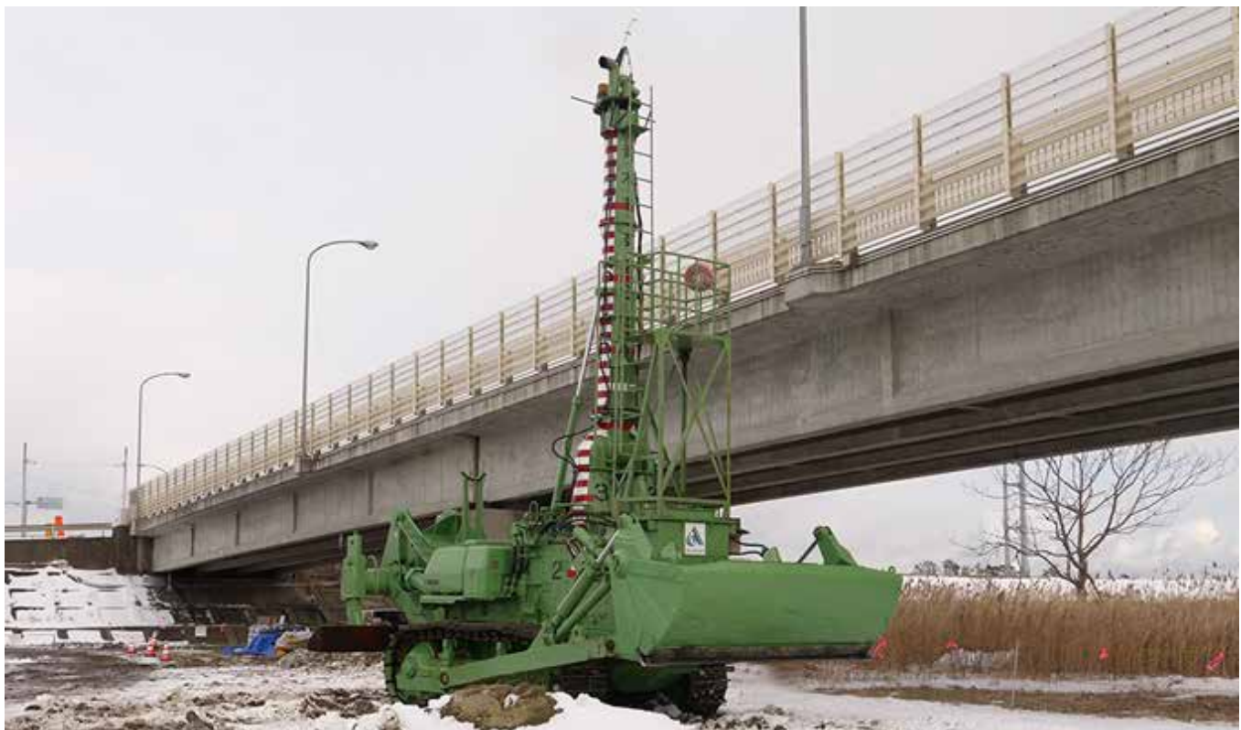
●● Amphibious bulldozer in operation in the Natori River in Miyagi Prefecture
