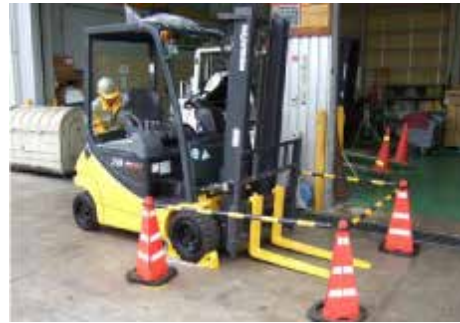
●● Cone barriers are set up to ensure safety during work at customer sites.
