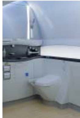
Lavatory equipped with Washlet
