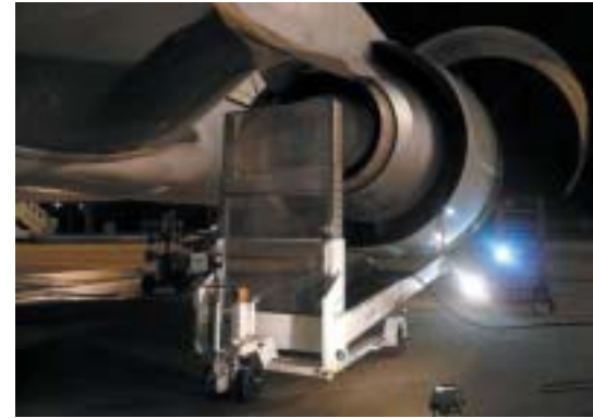
Washing the engine compressor
