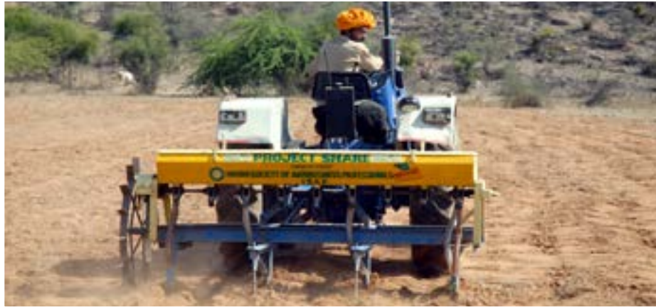
Jamuna Lal, Indian farmer, using a new sowing and fertilizing drill that revolutionized his farming practice.
