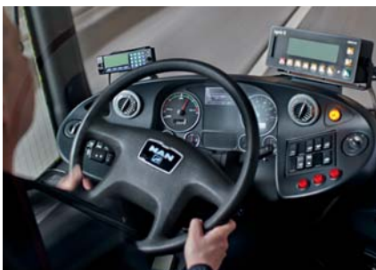
An additional display keeps the driver informed about the status of the high-capacity condensers on the roof.
