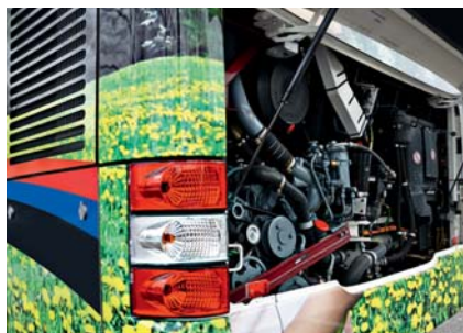
The eco-friendly MAN diesel engine starts generating electricity as soon as the stored braking energy is used up.
