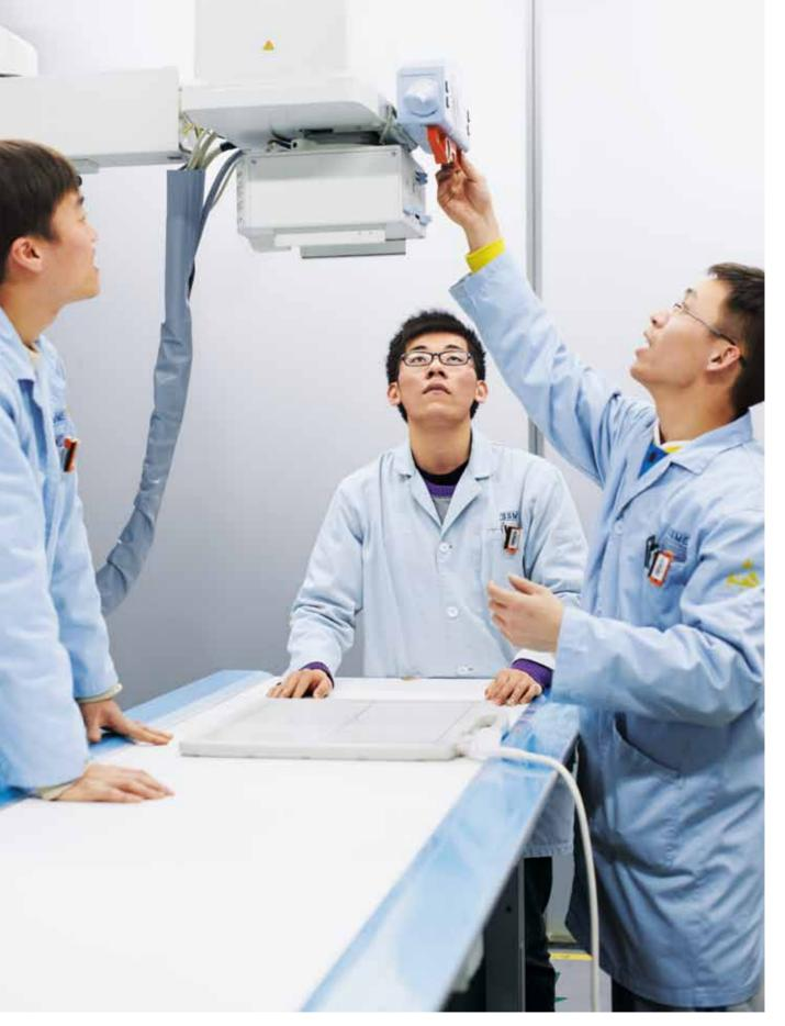
ABOVE – Before delivery our engineers inspect the technical reliability and image quality of the Multix Select DR. The mobile X-ray detector can be seen on the X-ray table.
