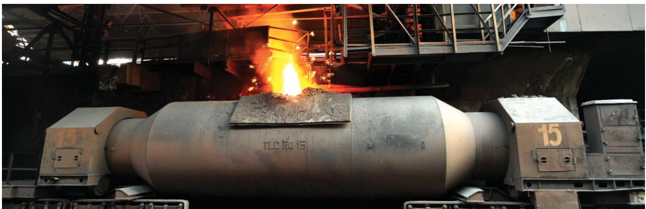
Torpedo ladle cars ensure energy efficient transfer of hot metal
