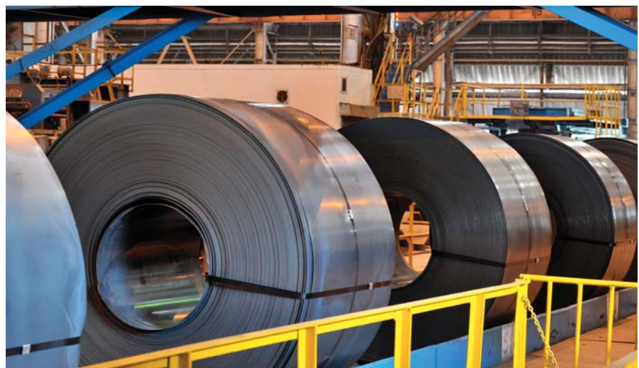
After Quality Inspection Cold Rolled Coils are ready for despatch at the Steel Works
