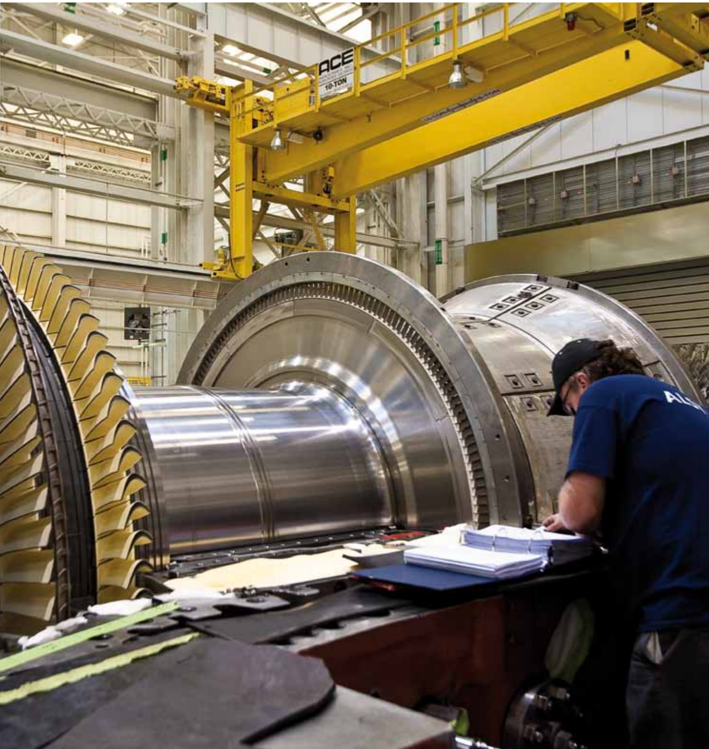
The first next-generation GT24 gas turbine, manufactured at the Chattanooga site (USA), offers enhanced operational flexibility.
