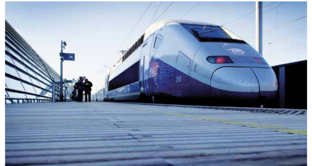
TGVs (shown above, a TGV Duplex) now operate at higher speeds than their predecessors, without any increase in noise levels.
