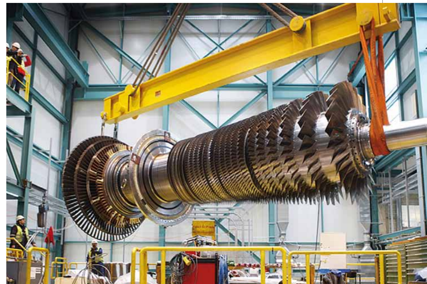
Workers test a GT26 gas turbine.
