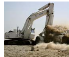
Hitachi Construction Machinery's land mine removal excavator
