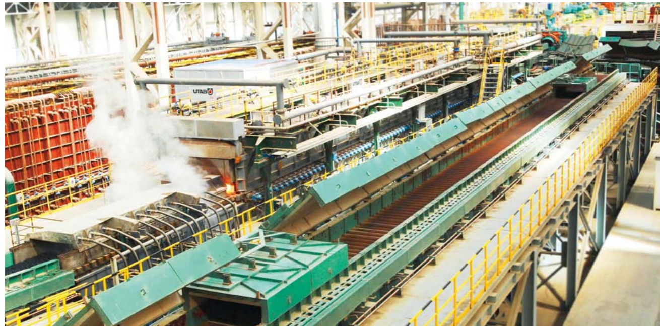
国内首台在线固熔炉 China's first in-line solution heat treatment furnace
