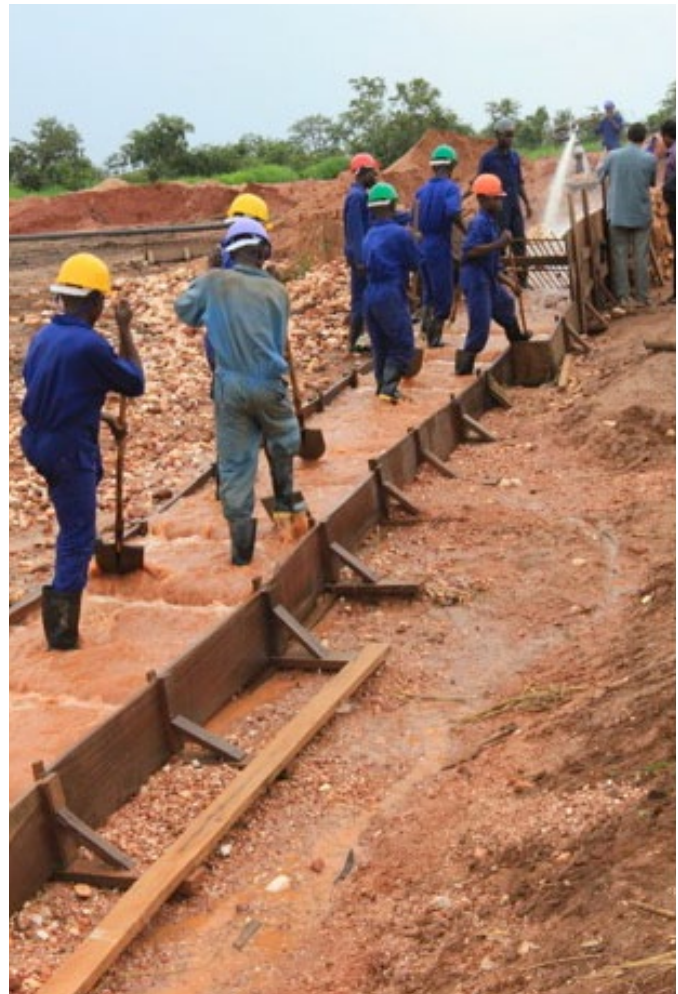
Miners using a sluicing technique to concentrate tantalite ore at the Mai Baridi Mine in Katanga.
