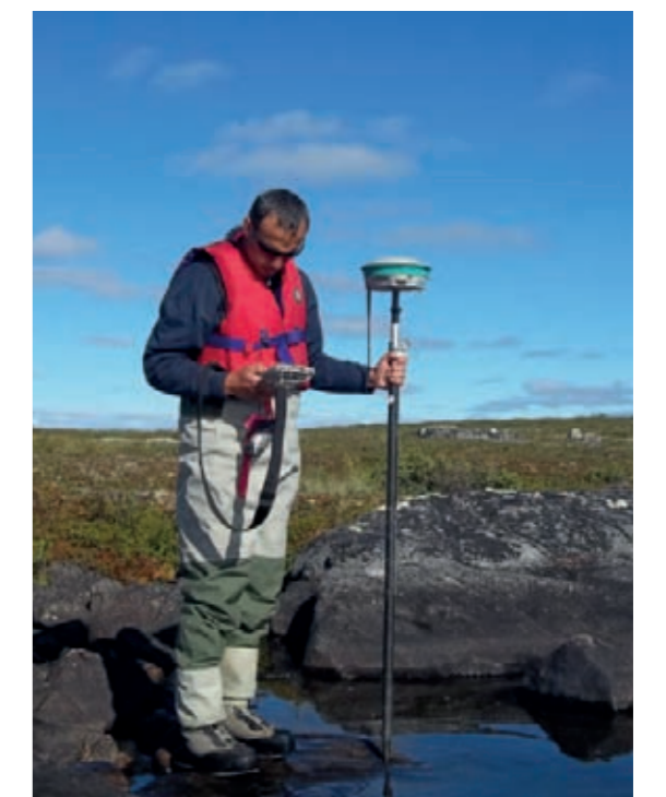
Measuring the water level near the Gahcho Kué project site, Canada.
